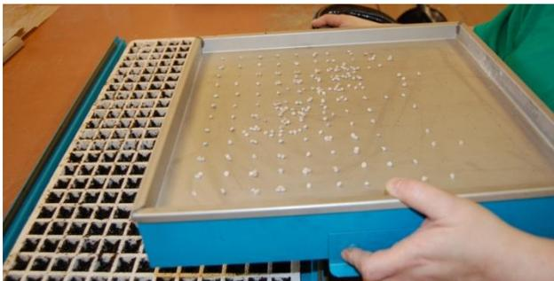
Figure 2. Pelleted seed being spread on a vacuum seeder.
